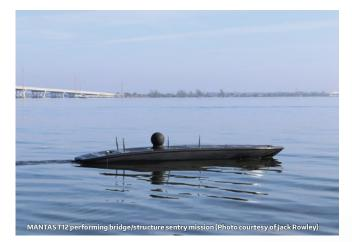
For underwater imaging, the MANTAS could be equipped with Norbit iWBMS STX multi-beam sonar, a forwardlooking sonar, side-scan sonar, or other commercial-offthe-shelf underwater sensors that can image underwater piping and bottom structures. This technology is in high demand to inspect commercial dams, energy plants, canals and other structures.
