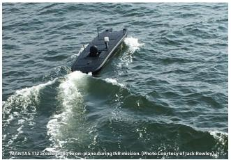
a MANTAS USV was used to conduct inspections of the Keokuk dam and energy center, the Bagnell energy center, the Elkhart hydro dam, the Central Arizona Project canal and other infrastructure.
