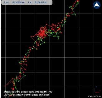
As shown on the graphics, Gaps USBL and the two transponders were able to successfully track the ROV at great depths during the whole duration of the operation with high repeatability of the position within 2 meters. It was furthermore estimated that iXblue's Gaps maximum tracking range could have reached 7,000 meters in the conditions encountered during the operation.
